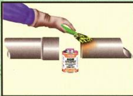
5. Apply one even coat of AGM cement to both of the surfaces to be joined, stroking the cement along and not around the surfaces. Do not apply excessive cement.
