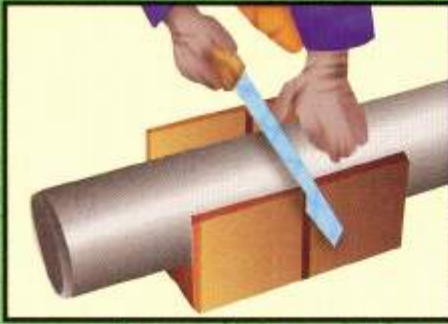
1. In the case of a pipe cut on site, cut the spigot end square.
