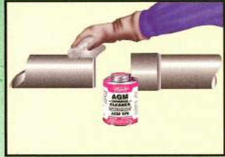
4. Clean the spigot and socket by using a clean dry cloth and AGM cleaner.
