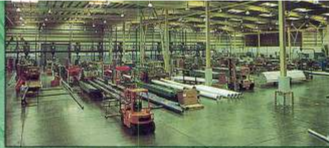
Production area with fifteen extruder machines.
